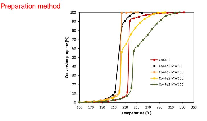
Propylene oxidation: Influence of the temperature during microwave irradiation C. Abou Serhal S. Siffert, R. Cousin, et al.
