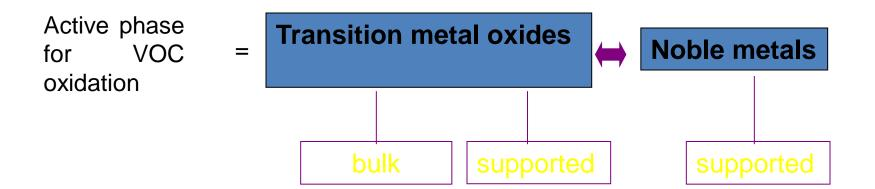
\* The support better dispersion of the active phase support-metal interaction mechanical strength thermal resistance...
