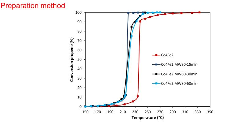
Propylene oxidation: Influence of time exposure to microwave irradiation C. Abou Serhal S. Siffert, R. Cousin, et al.
