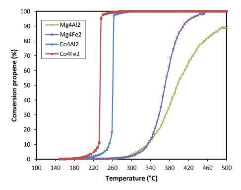
Propylene oxidation:  $Fe^{3+} > Al^{3+}$  $Co^{2+} > Mg^{2+}$  C. Abou Serhal S. Siffert, R. Cousin, et al.
