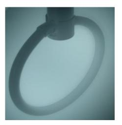
ICP plasma around a copper coil located inside the chamber
