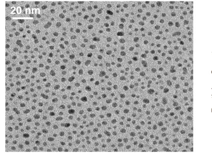
250 Mean diameter = 4.1 nm Std = 2.9 nm200 Particles Counts 150 100 50 0 8 9 0 2 3 5 6 10 Particle Diameter (nm) Adequate size for attractive chemical and
