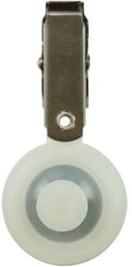
Back of VOC Chek 575 Sampler designed for easier analysis
